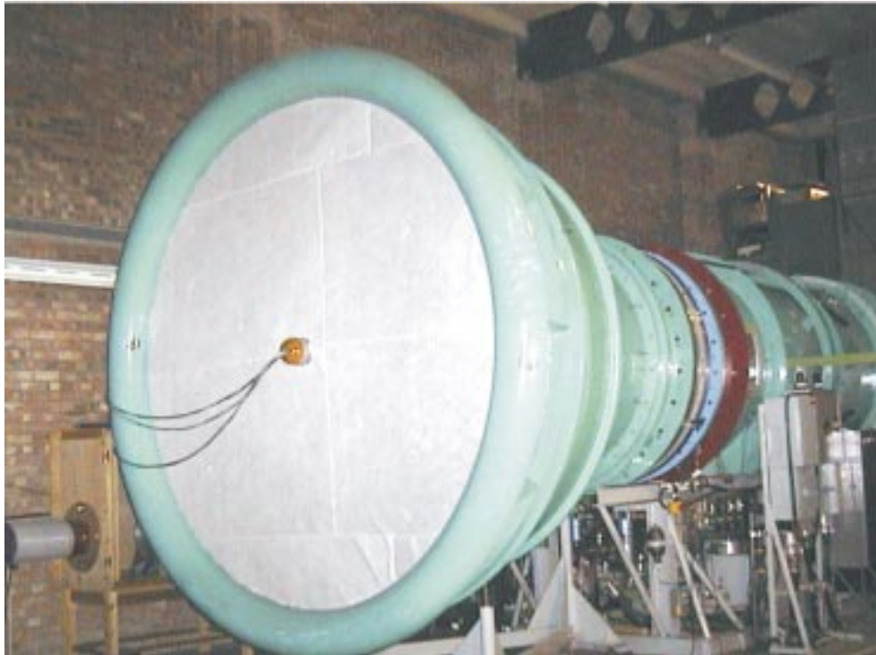
Figure 3.1(a) The low speed rotating turbine test facility
