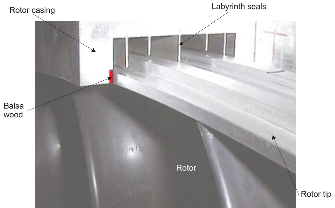
Figure 3.4 Rotor shroud arrangement
