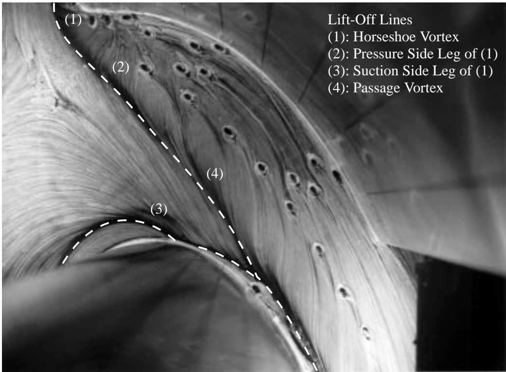
Fig. 129: Oil and Dye Surface-Flow Visualisation on the Film-Cooled Endwall at an Inlet Blowing Ratio of M_{inlet} = 2.0
