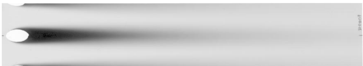
Fig. 46: Scanned Coolant Traces on a Diazo Coated Flat Plate
