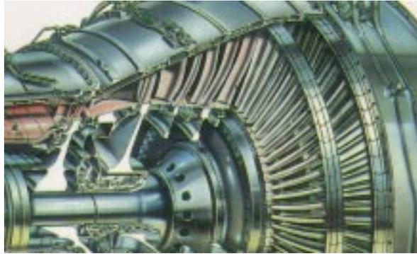
**Fig. 1 Rolls-Royce Trent 800 LP turbine.**
