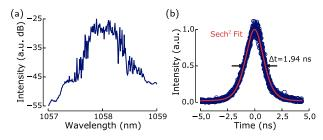
Fig. 4. Pulse characteristics at output of the circulator when the oscillator is operating in a noise-burst regime: (a) spectrum and (b) streak camera trace.
