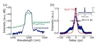
Fig. 3. Compressed pulse characteristics: (a) spectrum and (b) autocorrelation trace with streak camera trace inset.
