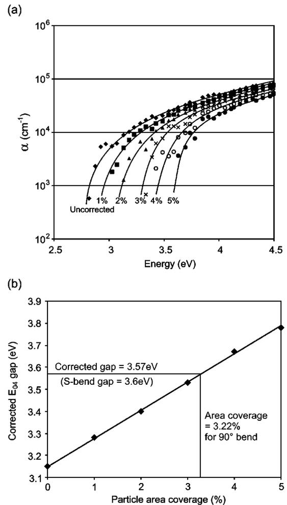
FIG. 5. (a) Corrected optical absorption coefficient ( $\alpha$ ) vs energy plots are derived for the 90°-bend filter film by taking into account various particle area coverages (1%–5%). (b) The  $E_{04}$  gap is plotted against the particle area coverage. For 3.22%, which is the particle area coverage of the 90°-bend filter film, the corrected gap of 3.57 eV corresponds well to the gap of the clean S-bend filter film of 3.6 eV.
