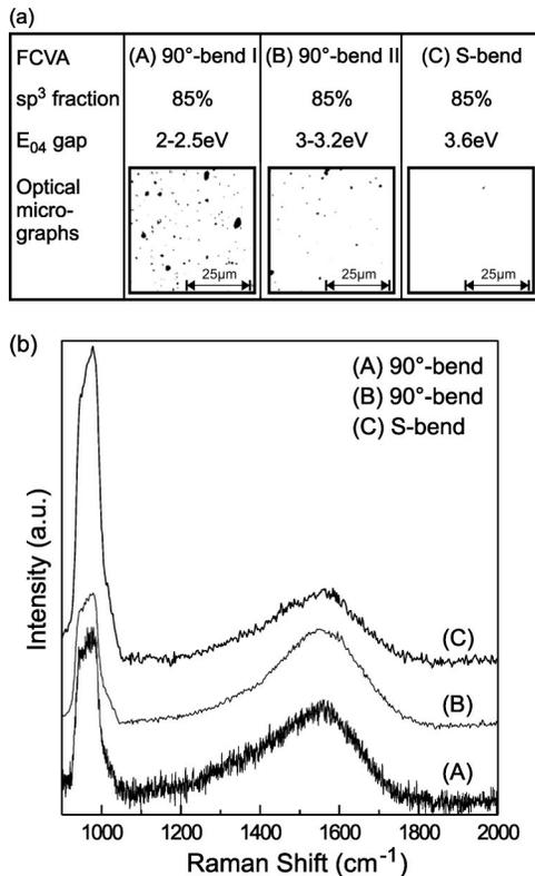
FIG. 1. (a) *ta*-C films produced from FCVAs with different filters can have the same *sp*<sup>3</sup> content in the matrix but different measured optical *E*<sub>04</sub> gaps. (b) Raman spectroscopy shows that there is little or no clustering (lack of D peak) in the *ta*-C matrix. It is clear that the microparticle inclusions affect the optical gap measurement since the *ta*-C matrix in all three cases is essentially the same.
