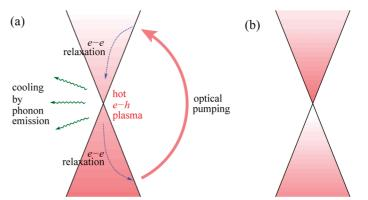
Figure 2. Schematic illustration of photoexcited electron kinetics in graphene. The intensity of the color shading represents the electron population, in the case of (a) efficient interband relaxation and (b) inefficient interband relaxation.
