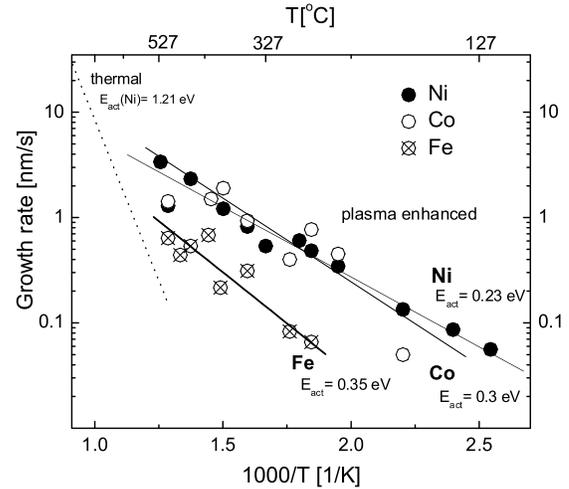
FIG. 2. Arrhenius plots for CNF growth rates on different catalysts in  $NH_3$  diluted  $C_2H_2$ . The activation energies are calculated from the slope of the linear fit to the data. Temperature dependent changes in the CNFs crystallinity are not considered. The dotted line is the growth rate variation for Ni thermal CVD ( $E_{act} = 1.21$  eV [11,42]).
