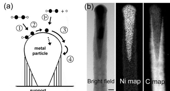
FIG. 1. (a) Schematic of the growth process. (b) Bright field image and electron energy loss spectroscopy Ni *L* edge (854 eV) and carbon *K* edge (284 eV) elemental maps of a PECVD CNF at 500 °C. Scale bar: 20 nm.
