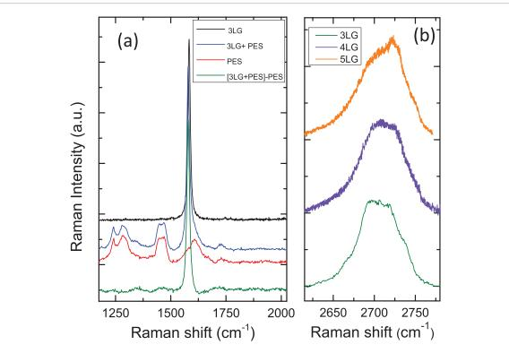
**Figure 3.** (a) Raman spectrum measured at 514 nm for a 3LG device, before (black) and after (blue) PES drop-casting, together with the Raman response from the PES (red) and the spectrum with the subtracted background (green). (b) Raman 2D region for 3LG (green), 4LG (violet) and 5LG (orange).
