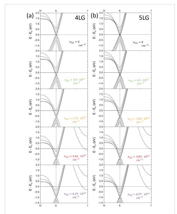
**Figure 5.** Band structure evolution with increase of doping in 4LG (a) and 5LG (b), for selected values of  $n_{2d}$ . For  $n_{2d} \lesssim 2 \cdot 10^{14}$  cm<sup>-2</sup>, the effect of the extra carriers is comparable to a rigid-band shift. Larger doping induces new structures.
