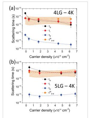
**Figure 7.** (a)  $n_{2d}$  dependence of  $\tau_{\varphi}$  (black dots),  $\tau_i$  (red dots),  $\tau_{tr}$  (blue dots) and  $\tau_{\varphi}|_{e^{\bullet}e^{\bullet}}^{e^{\bullet}e^{\bullet}}$  (orange dots and shaded band) at 4 K in 4LG; (d) The same as in (a) but for 5LG. Dashed lines act as guides to the eye.
