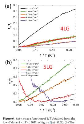
**Figure 6.** (a)  $\tau_{\varphi}/\tau_i$  as a function of 1/T obtained from the low-T data (4 < T < 20 K) of figure 2(a) (4LG); (b) The same as in (a) but for the low-T data of figure 2(d) (5LG). Dashed lines are fits to the experiments according to equation (8). Best fits for 4LG are omitted for clarity.
