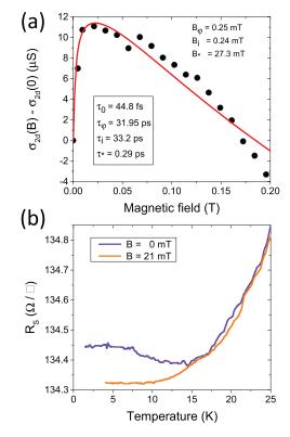
**Figure 4.** (a) B dependence of conductance relative to the value at zero field (black circles) and fit by using equation (2) (red solid line) for 3LG. (b)  $R_S$  as a function of T for the 3LG device of figure 4(a) for B = 0.021 T and 0T.
