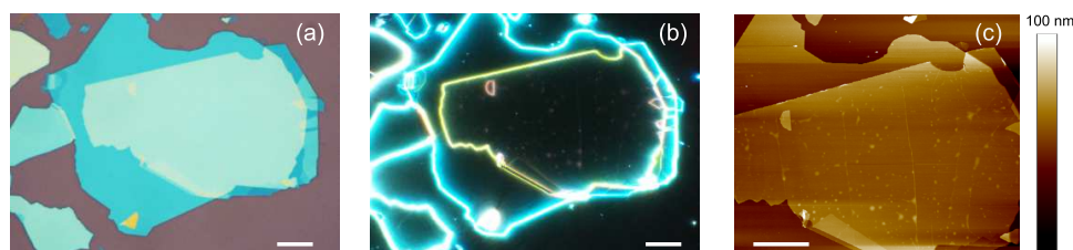
Figure 3. (a) Bright field, (b) dark field, and (c) AFM images of SC-SLG encapsulated in hBN. Scale bars: 10 \mu\text{m} .
