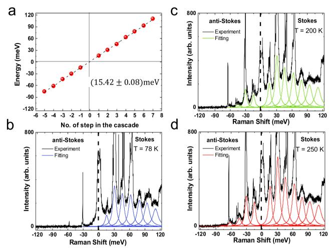
Fig. 2 Energy separation and T dependence. a Emission energies as a function of number of steps in the cascade, extracted from the RT spectrum in Fig. 1b. The dashed black line is a linear fit, giving a step energy -15.42 ± 0.08meV. b-d 532 nm Hot PL spectra of 1L-WSe<sub>2</sub> at b 78 K, c 200 K, d 250 K.
