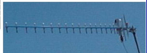
Superposition effects result in a highly directional wave as long as the spacings (a,b) and the phases ( $e^{j\alpha}, e^{j\beta}$ ) are correct
