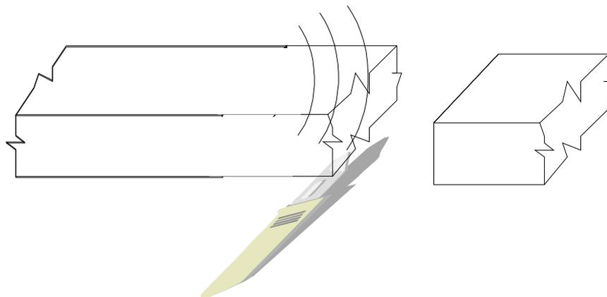
The electromagnetic waves in a guide will radiate if you chop its end off (very inefficient)
