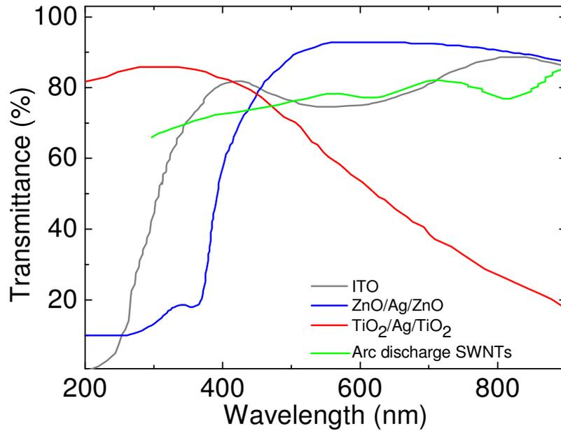
Metal grids, metallic nanowires, metal oxides and nanotubes (SWNTs) have been explored as ITO alternative
