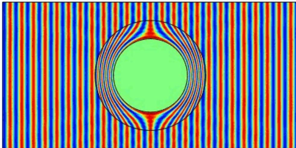
The plane wave impinging from left is "flowing" around the cloak without being disturbed by the metallic cylinder in the middle **210**
