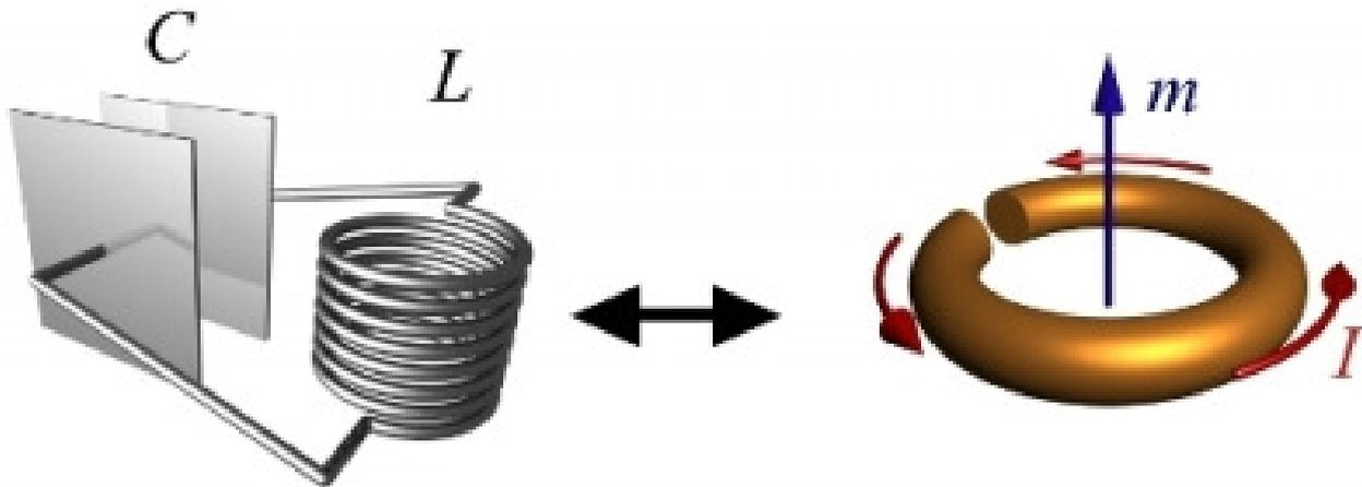
SRR act as  $LC$ -oscillators. Since the capacitance and inductance are determined by the dimensions of the SRR, scaling of the structure allows to tune the resonance frequency from microwave to terahertz to the infrared
