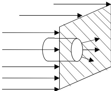
A laser can be thought of as an aperture antenna and the output roughly approximates to a plane wave.
