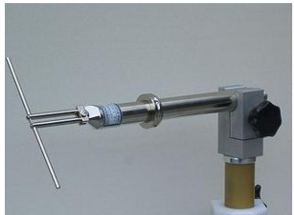
GHz half-wave dipole Antenna
