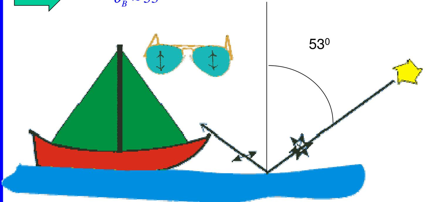
A rule of thumb: polarized filters limit the glare from calm waters for a sun altitude between 30 and 60 degrees
