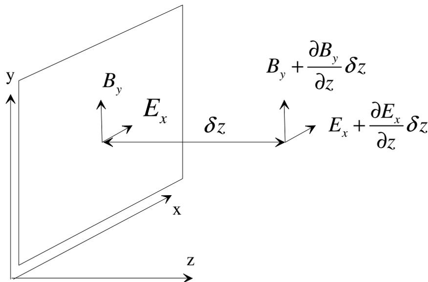
In the plane  $z = \delta z$ , the fields will have varied by the rates of change of  $\underline{B}$  and  $\underline{E}$  with  $z$
