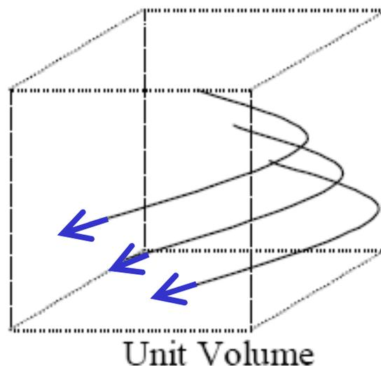
**Strength** of the field = **Number** of flux lines per unit area
