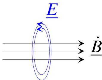
The Maxwell-Ampere Law  $\oint_c \underline{H} \cdot d\underline{l} = \int_s (\underline{J} + \dot{\underline{D}}) \cdot d\underline{S}$
