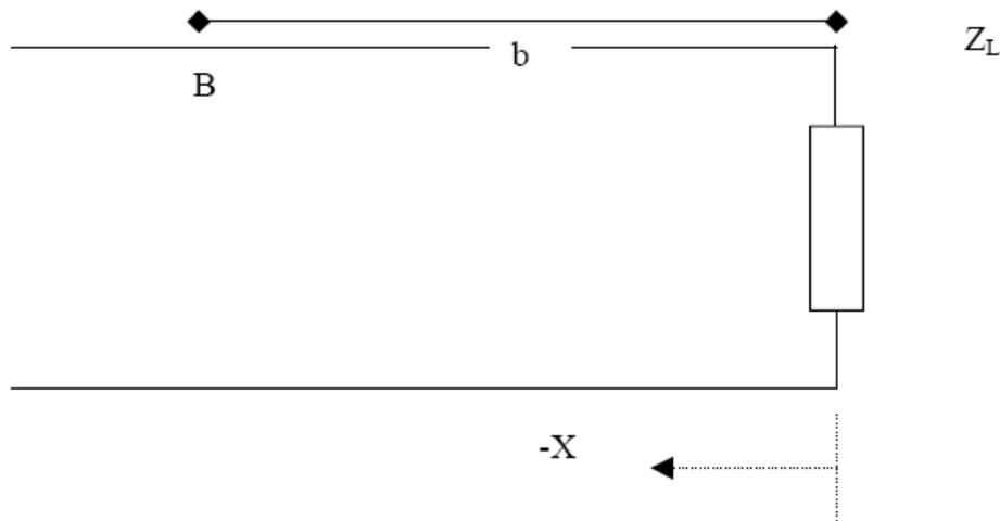
The impedance of a line is  $Z_0$  only in the absence of reflections. With reflections the impedance at point B is a function of:
