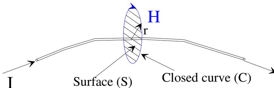
Note: since the field strength comes from the total current flowing, this explains how coaxial cables shield fields
