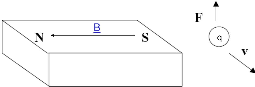
A charge **moving** with velocity  $\underline{v}$  in a magnetic field also experiences a force
