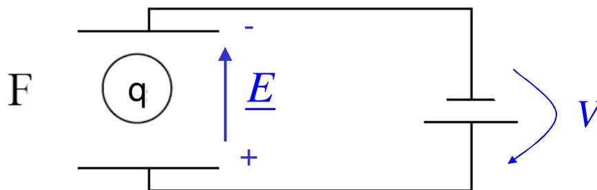
A charge  $q$  placed in an electric field experiences a force  $\underline{F}$  which is dependent on the charge itself and on the electric field strength  $\underline{E}$
