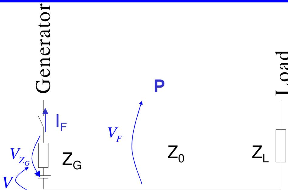
1. At switch-on, a pulse  $V_F$  is generated and travels towards the load
