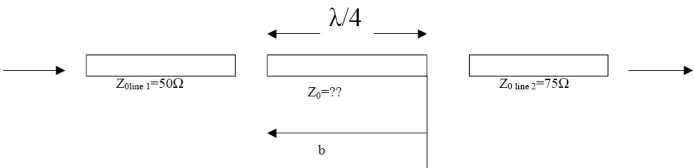
Second line appears as  $Z_L = Z_{0\text{Line2}} = 75 \Omega$  to the  $\frac{1}{4}$  wave link
