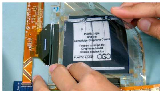
Active matrix electrophoretic display incorporating graphene. Credit: University of Cambridge
