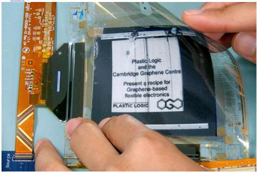
The world's first flexible graphene display has been created by UK researchers, paving the way for printable, foldable electronics. The display developed by the Cambridge Graphene Centre and Plastic Logic, a spin-off company from Cambridge University, is similar to electronic paper used in today's e-readers. The main difference is that it's made of flexible plastic instead of glass and that it incorporates graphene in its pixels.
