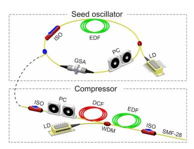
With fibre lasers, femtosecond pulses are typically generated through soliton mode-locking. A soliton is a self-reinforcing solitary wave that maintains its shape without distortion as it travels at constant velocity along a waveguide such as an optical fibre. Solitons are the result of dispersive and nonlinear effects that cancel each other out in the waveguide medium, thereby allowing a stable pulse envelope to propagate.
