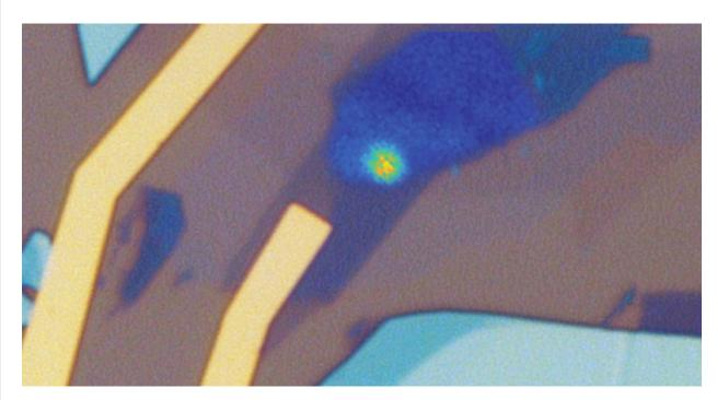
An overlay of the microscope image of a quantum LED device and the photoluminescence image from the active area of WSe2. The isolated bright spot corresponds to a quantum emitter generating a stream of single photons. Image credit: Mete Atatüre
