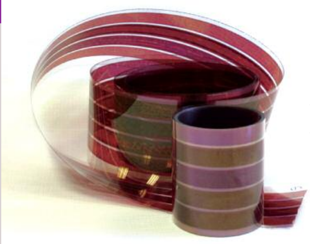
Solar cells can now be manufactured by roll-to-roll printing
