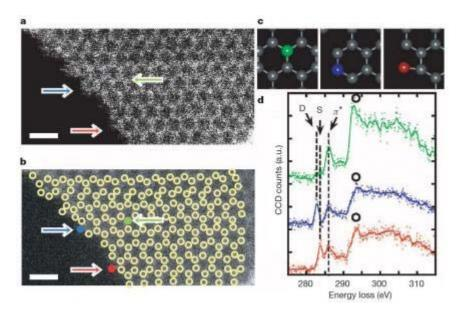
Characterising individual atoms of graphene. The atoms depicted in red, blue and green colours represent atoms at different positions on a graphene sheet. Their energy loss spectra mirror their different properties. Reprinted by permission from Nature doi: 10.1038/nature09664 (2010).
