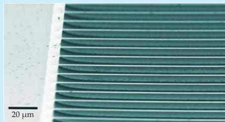
order of magnitude, arises primarily from the larger difference in thermal expansion coefficients and from the Al beam’s smaller initial tension compared with that of the Au–Pd beam. With their high quality factors, microresonator-based sensors would potentially have exceptional temperature resolution as well. (A. K. Pandey et al., *Appl. Phys. Lett.* **96**, 203105, 2010; T. Larsen et al., *Appl. Phys. Lett.* **98**, 121901, 2011.) —RJF
