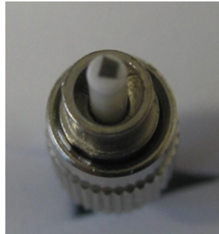
Optical Fibre End with Nanotube Polymer Composite Mode-locker
