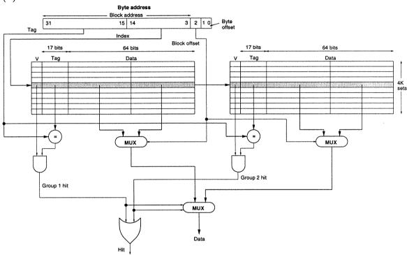
Compared with the direct-mapped case, there is an extra multiplexor at the output (to select between different blocks in each set) which will have a finite propagation delay and therefore increase the hit time.
