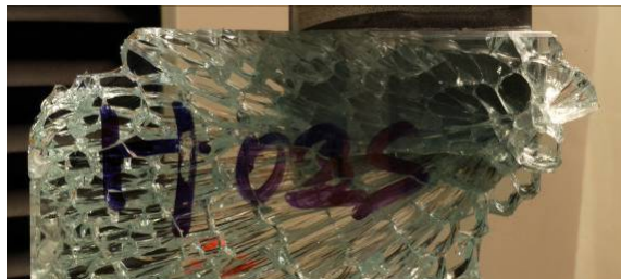
Figure 5 - Glass Failure in Glass-Steel tests
