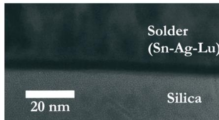
Figure 1 High-resolution TEM micrograph showing the nanometer-scale bonding layer (darker band at silica-solder interface) [2].
