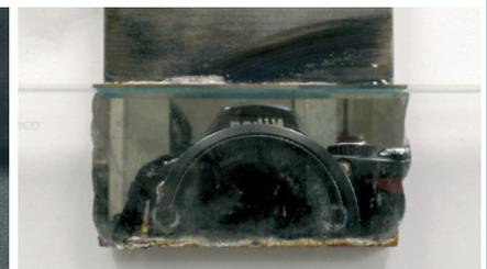
Figure 2 The "mirror-finish" of a soldered glass-steel joint aided by the use of ultrasonic vibrations
