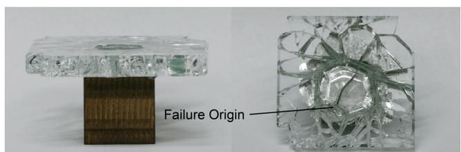
Figures 6a and 6b "Fully toughened" failure mechanism for the cube pull-off tests
