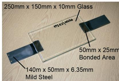
Figure 8 The single lap shear specimen
