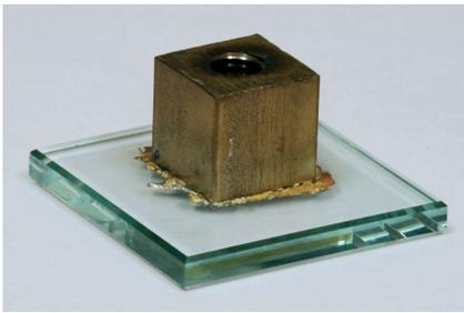
Figure 3 A typical sample from the cube pull-off tests.
