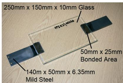
Figure 8 The single lap shear specimen
