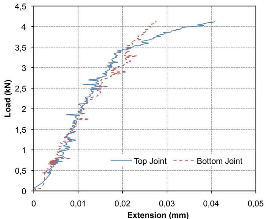
Figure 9 Experimental results from the single lap shear test
