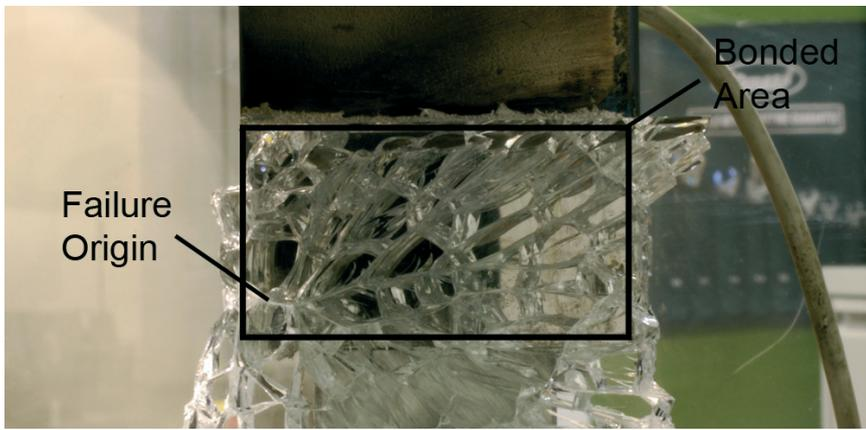
Figure 10 Origin of failure of single lap shear sample
