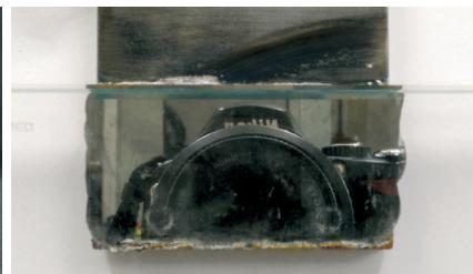
Figure 2 The "mirror-finish" of a soldered glass-steel joint aided by the use of ultrasonic vibrations
