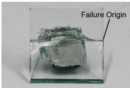
Figure 7 “Annealed glass” failure mechanism for the cube pull-off tests
