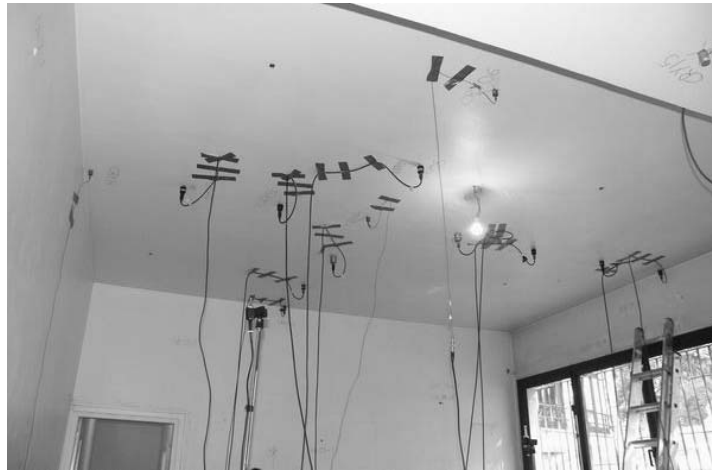
Fig. 3. The measurement site in the basement with accelerometers on the ceiling.
