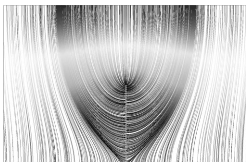
Figure 2. Simulated electrical field profile surrounding the single carbon nanotube (10 \mu\text{m} high) with an applied field of 1\text{V m}^{-1} .
