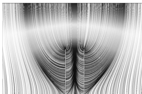
Figure 3. Electric field profile of a two-nanotube electrode, 1\text{ }\mu\text{m} apart at 1\text{V m}^{-1} .
