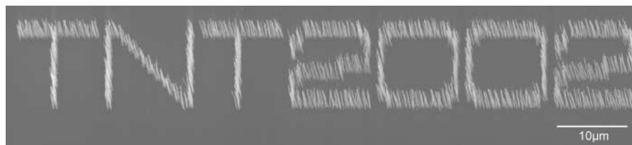
Figure 1 The conference logo writ small. Carbon nanotubes such as these could make both the computers and displays of tomorrow. (Image courtesy Kenneth Teo, Manish Chhowalla, Gehan Amaratunga and Bill Milne, Univ. Cambridge.)
