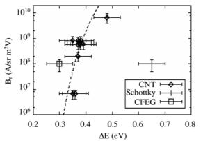
**Fig. 3** Field emission brightness,  $B_r$ , as a function of the energy spectrum,  $\Delta E$ , for several MWCNTs. Data for a Schottky emitter and a tungsten cold field emission gun (CFEG) are also included [6].
