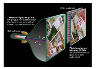
**Fig. 5** (online colour at: www.pss-a.com) Schematic of a CRT (uses a thermionic emitter) and FED (uses an array of cold cathode emitters).
