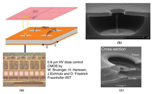
**Fig. 7** (online colour at: www.pss-a.com) a) Schematic of the e-beam lithography system, b) gated CNT, c) cross section of the electron gun.
