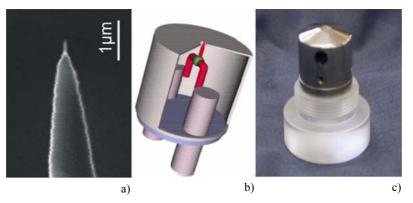
**Fig. 2** (online colour at: www.pss-a.com) a) MWCNT on top of a tungsten needle, b) how the tungsten needle is integrated into the electron gun module, c) complete gun ensemble.
