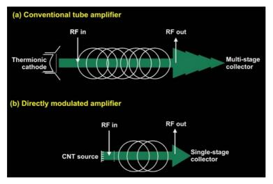
**Fig. 4** (online colour at: www.pss-a.com) a) Conventional travelling wave tube, b) directly modulated CNT based TWT.
