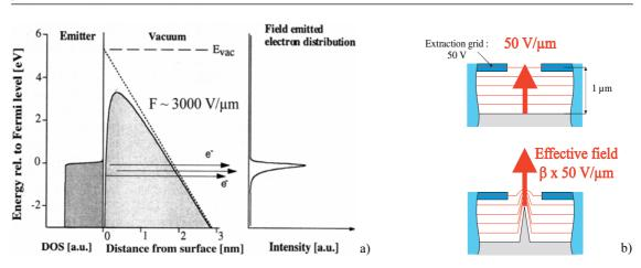
Fig. 1 a) Process of field emission, b) (online colour at: www.pss-a.com) field enhancement.
