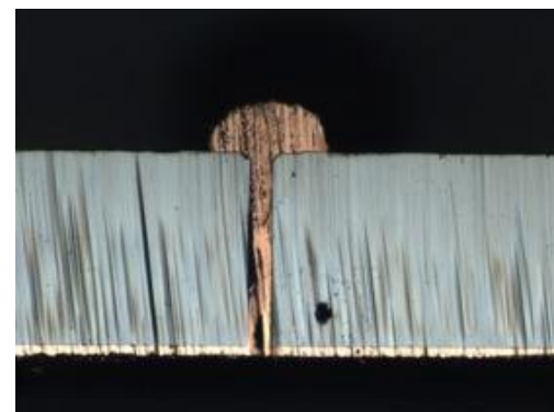
Section through a plated via
