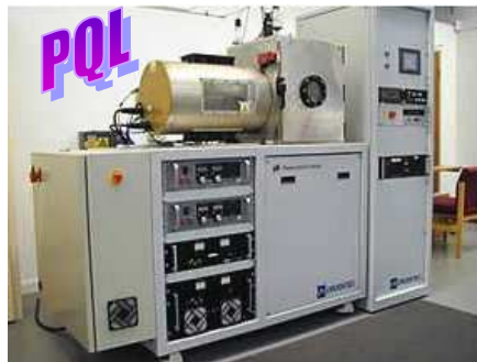
Plasma Quest HiTUS sputter deposition of TCO at low temperature
