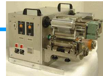
Yasui Seiki Microgravure Coater for printing polymer films for PV
